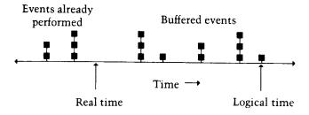
Event buffering can reduce or eliminate timing inaccuracy. As an example, suppose a composition program uses 0.2 CPU sec to compute each note and that most notes are 1 sec apart, but occasionally there is a burst of 10 notes only 0.1 sec apart. If the CPU can buffer 2 sec of notes, it is able to keep ahead of schedule, allowing accurately timed event performance.
